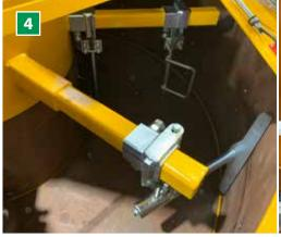
Mixing arms and side scrapers Adjustable mixing arms and side scrapers in steel and hard PUR. Equipped with safety bolts to prevent large stones from seriously damaging the mixing arms. The adjustability makes sure that any concrete is mixed homogeneous and without lumps.
