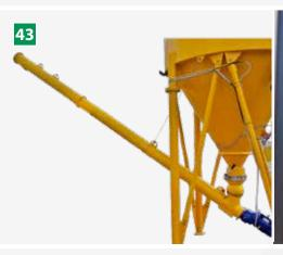
43 Cement auger with gearbox (optional) Available in several lengths. All augers are complete with either flange or universal ball joint inlet, flange for butterfly valve, cylindrical outlet, and service hatch under the inlet.
