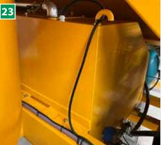
23 Insulation/Winter package 2 (optional) This package includes all items from winter package 1, and, as an extra feature, the tank is insulated with 45 mm insulation material. Note! The water heater is not included and must be ordered separately if water needs to be heated.
