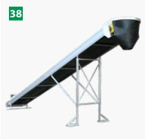
Hydraulic Belt conveyors (optional) Belt conveyors with belt widths of 0.8 m and lengths of 6 m - 14 m. With hydraulic system for automated operation of adjustusting the heigh. All conveyors are equipped-with a drum motors, integrated gearboxes, inlet boxes, dispenser funnels, and lifting hooks for easy transportation.
