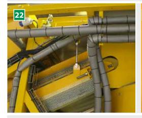
22 Insulation/Winter package 1 (optional) Liquid supply lines are equipped with trace heating tape and additional insulation. The cabinet for additive and high-pressure cleaner pumps is fitted with a radiant heater.
