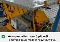
to protect aggregates from the elements. Easy and quick deployments with a manual winch. Including grid under cover to miniize water on the cover.
