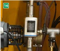
Flowmeter for additives (optional) Electromagnetic flowmeter, ½" in stainless steel, max. 16 bar, temperature -10 to + 70 ° C, minimum conductivity 20 μS / cm. The flow measurement guarantees a dosing accuracy of +/- 1 % (repeatedly +/- 0.2 %).
