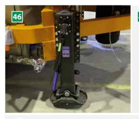
46 High extended support legs (optional) Set of high extended legs with a length of 0-5200 mm. Very useful for different placement sites and in connection with a concrete pump.
