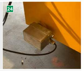
24 Water heater (optional) Electric heating in the water tank for frost protection. Complete with thermostat and switch. The heater is usually connected to the control cabinet for automatic operation and frost protection. Power 4 kW. Voltage 3 x 400 volts.
