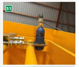
51 Level sensor for concrete pumps (optional) Level sensor for installation in concrete pumps.
