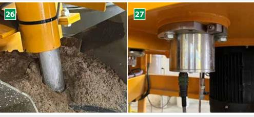
25 Temperature sensor for the water tank (optional) 26 Moisture sensor for hopper (optional) Sensor for measuring moisture in the dosed sand prior to entering the mixer. 27 Moisture sensor for the mixer (optional) Moisture sensor mounted in the mixer to indicate batch moisture level.
