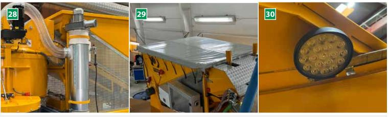
Dust filter for the mixer (optional) 28 Filter to reduce cement dust in the environment during the dosing process.
