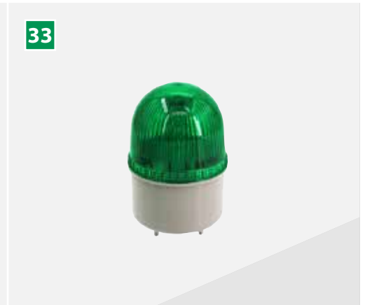
33 Alarm light (optional) Light activated when mixer has ended mixing time and concrete is ready for use.
