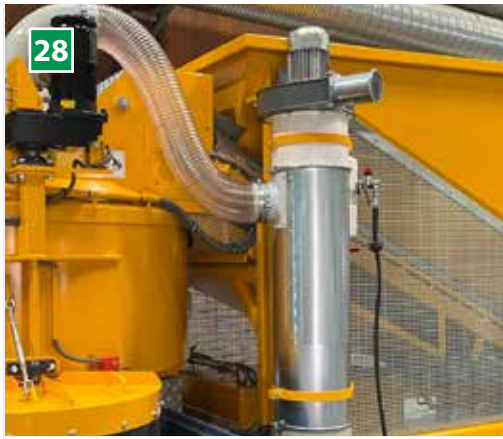
28 Dust filter for the mixer (optional) Filter to reduce cement dust in the environment during the dosing process.
