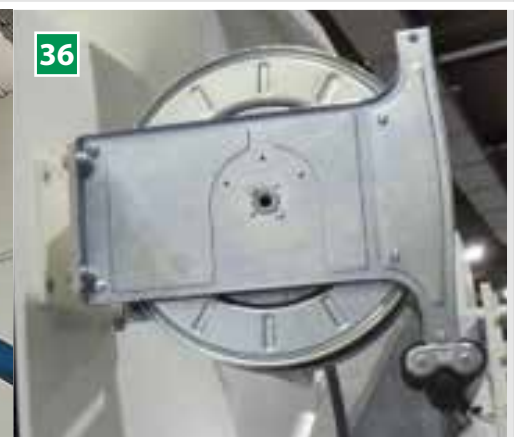
36 Hose reel (optional) Hose reel for easy reeling and storage of the hose for high-pressure cleaner
