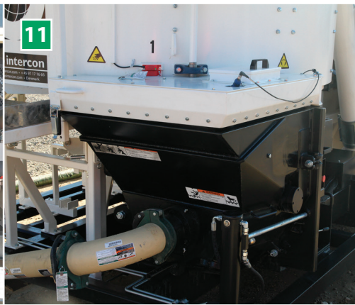
11 Concrete pump (option) The concrete pump is a stamp pump that is hydraulically controlled. Storage tank with full indicator, safety cover and a safety switch for cleaning. Storage tank approx 400 litres. Capacity 10 m 3 / hour. Conveyor distance max. 25 m.
