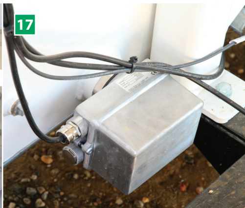
17 Water heater (option) Electric heating in the water tank for frost protection. Complete with thermostat and switch in control cabinet for automatic operation and frost protection. Power 4 kW. Voltage 3 x 400 volts, 50 Hz.
