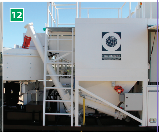
12 Cement container 2.0 m 3 (option) The cement funnel is equipped with full and empty detectors. The opening (1x1m) is intended for big bags. Seals for dust and moisture. A vibrator on the sidewall ensures that the material slips continuously.
