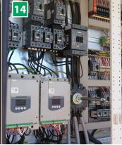
14 Frequent converter (optional) Frequent converter on mixer motor to achieve the perfect speed in the mixing sequence. The frequent converter can reduce the generator size by 25 %.
