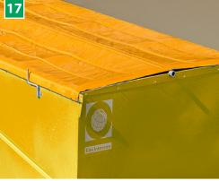
Water protection cover (optional) Removable cover made in heavy duty PVC, to protect material hopper from the elements and for easy cleaning of the material bunker.
