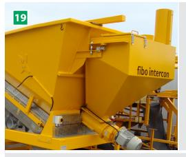
Preweighing of cement (optional) 19 Cement silo combined with cement auger. The equipment is suspended in weighing cells. The cement silo is supplied with a vibrator on the silo box and filter bag to reduce dust emissions when refilling. With the pre-weighing of cement, the dosage tolerance is +/- 1 % for the plant.
