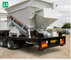
23 Trailer with twistlock system (optional) 40 feet trailer with 2 or 3 axles twinlock system. The trailer will ne delivered with 4 or 6 support legs.
