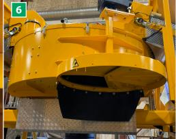
4 Mixing arms and side scrapers Adjustable mixing arms and side scrapers in steel and hard PVC. Equipped with safety bolts to prevent large stones from seriously damaging the mixing arms.
